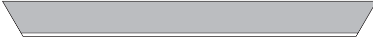
No. 80756.168 168,00 x 16 x 0,50 mm, einfasig, single bevel, simple biseau No. 80756.169 168,46 x 16 x 0,50 mm, einfasig, single bevel, simple biseau
