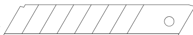
Snap-off blade 18 mm #180.050 and #180.051 109.4 x 18 x 0.50 mm, 180.051 with extra- broad, extremely sharp ground finish
